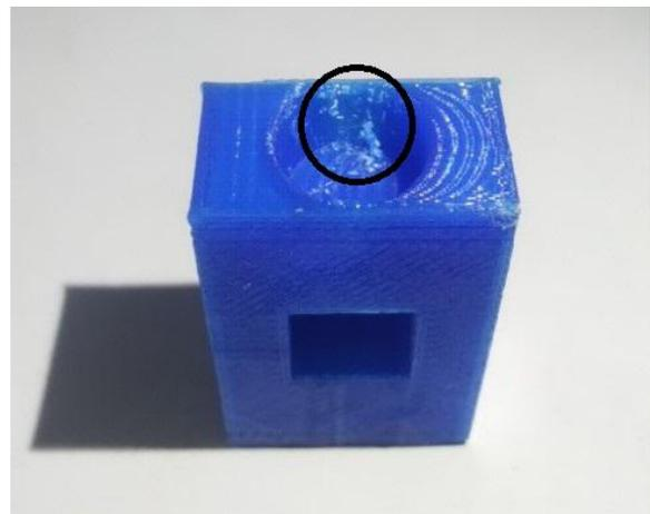
**Fig. - 7 :** Sample of Magnet Plate Printed Using FDM
