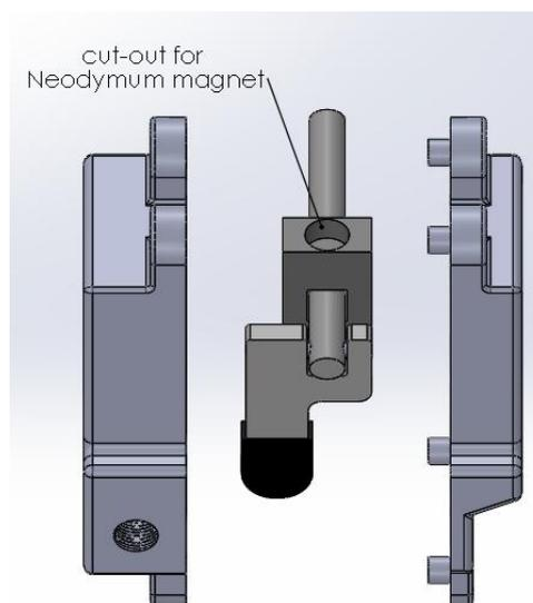
**Fig. -10 :** Depiction of Cut-out for Fitting Neodymium Magnet
