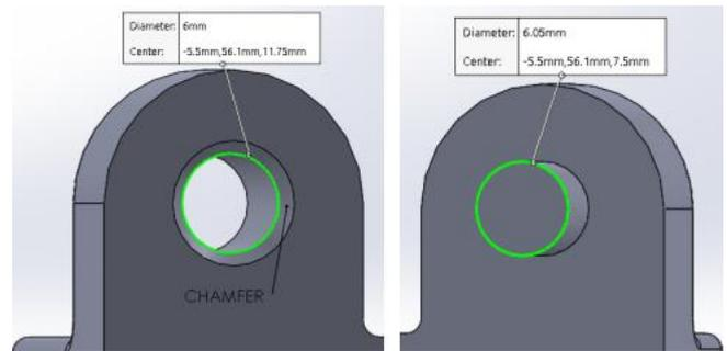
**Fig. - 6 :** Dimensions of Female & Male Parts After Tolerancing
