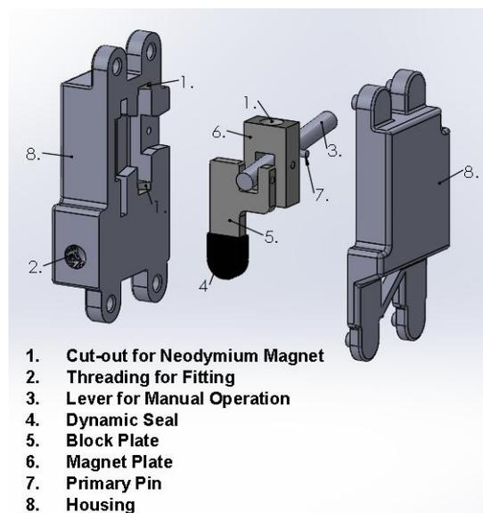
Fig. -1 :Exploded View of Assembly
