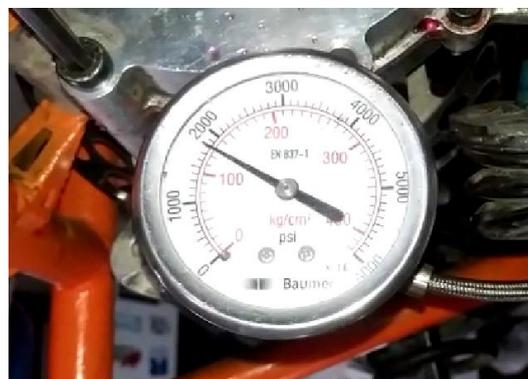
Fig. -5 : Hydraulic Pressure Gauge for Brake Line Pressure
